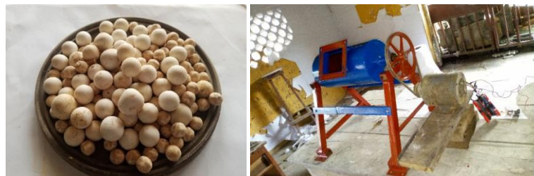
Figure 3a & b: Porcelain Pebbles of different sizes and Ball Mill (Ozidede & Ofili, 2024).
