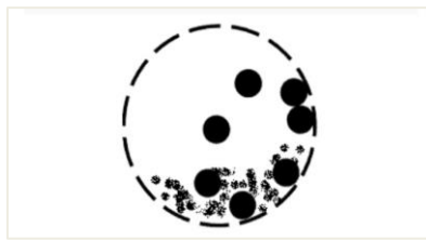
Figure 3c: Cascading effects of balls in a ball mill (source: http://en.m.wikipedia.org )
