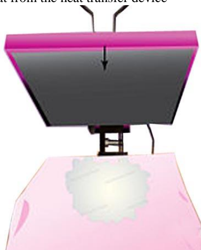
Fig 5. Application of heat from the heat transfer device
