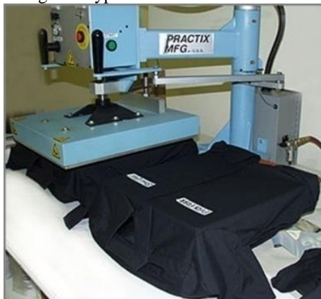
Fig 8. A typical heat transfer machine
